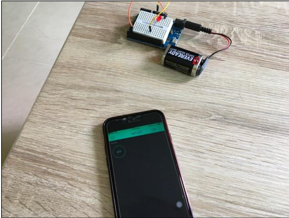
Using a smartphone to switch on/off an LED via WIFI
